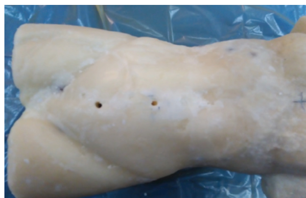
Figure 2. Location of the cylindrical ion chamber (Farmer)
