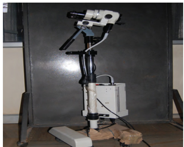
Figure 4. Carl Zeiss colposcope with a variable magnification index giving a magnification of approximately 6-20 \times .
