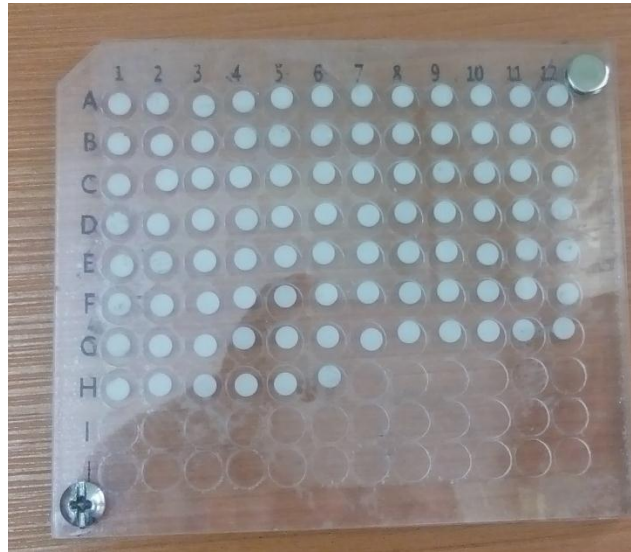
Figure 1. This figure depicts the TLD chips utilized in the present study. TLD: Thermoluminescent dosimeter
